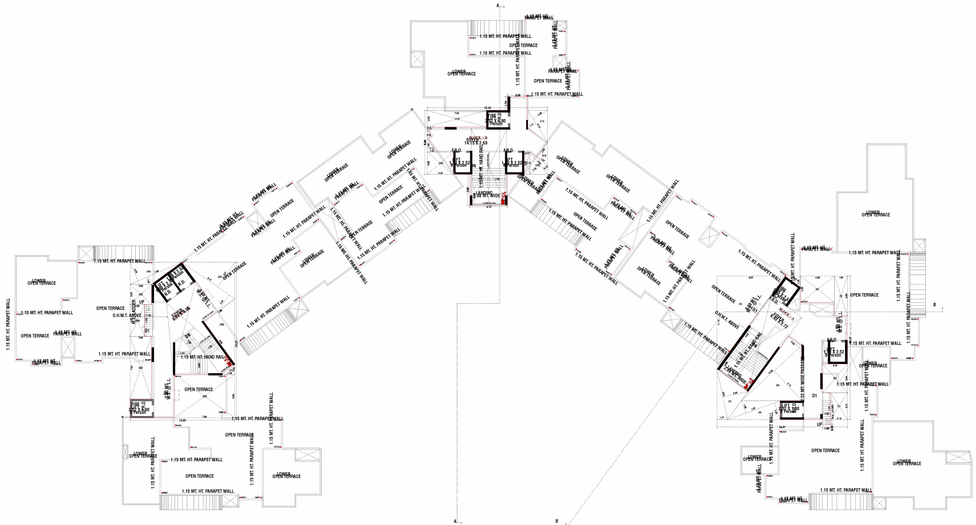
OPEN TERRACE PLAN (STAIR CABIN, LIFT MACH. ROOM & O.H.W.T.) NOTE :- ALL OUTER & INTERNAL WALL ARE OF 0.15 MT. TH. B/K WALL
