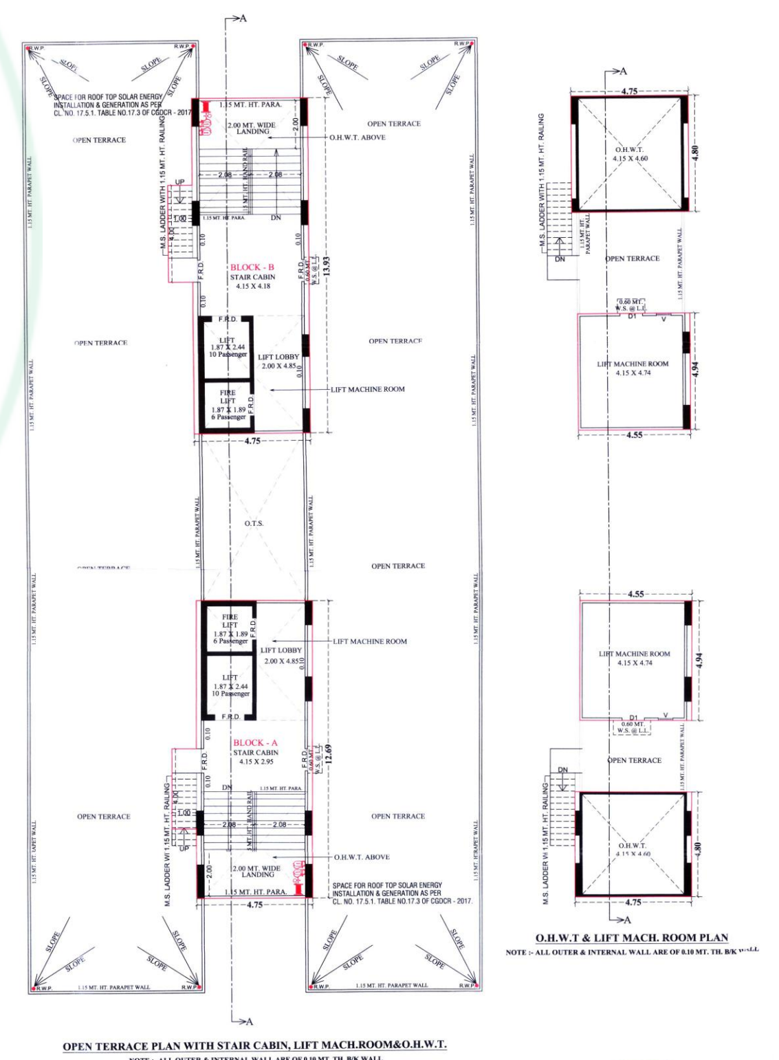
NOTE :- ALL OUTER & INTERNAL WALL ARE OF 0.10 MT. TH. B/K WALL.
