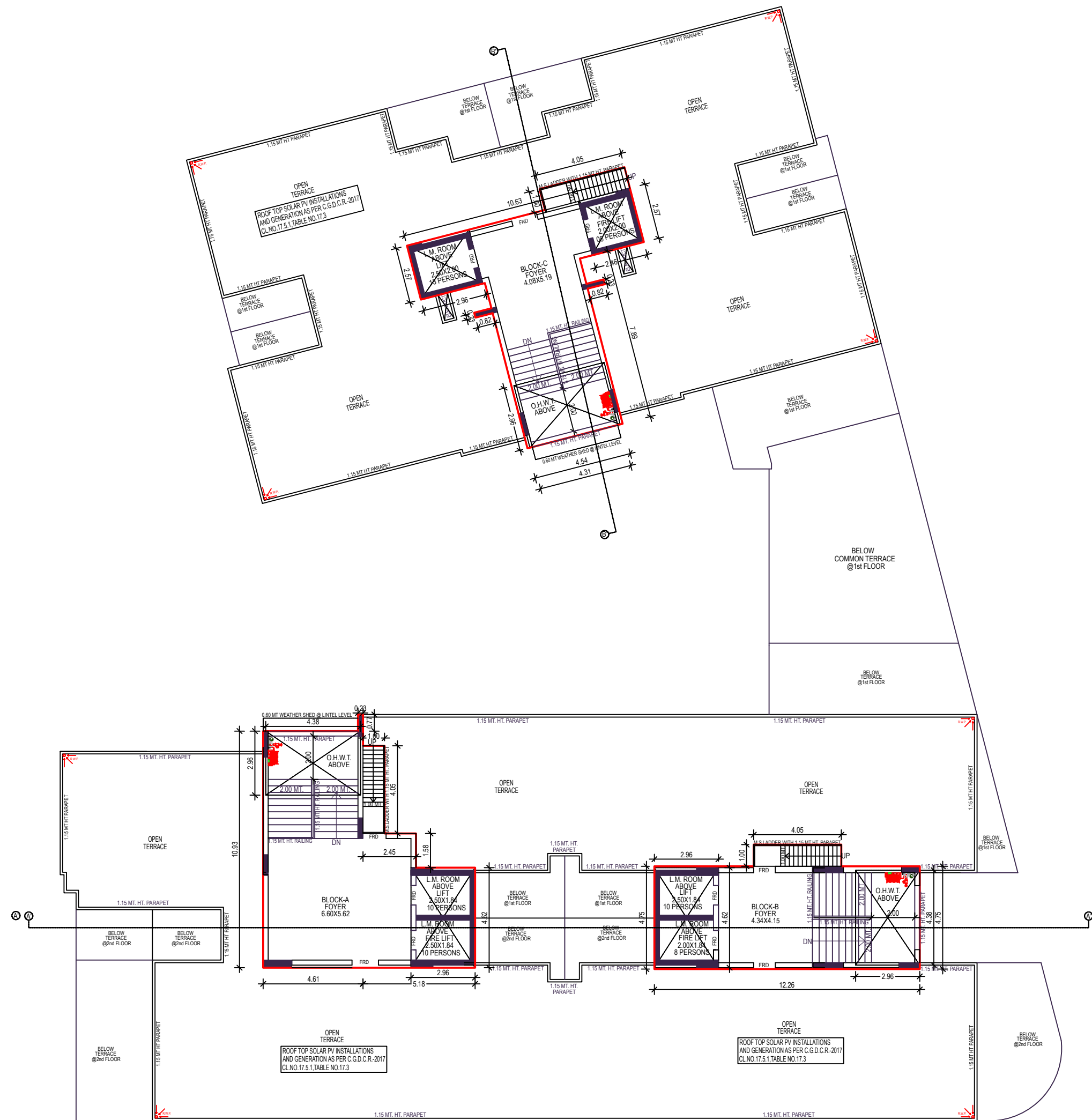
OPEN TERRACE PLAN WITH STAIR CABIN, L.M.R. & O.H.W.T.
