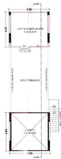
LIFT MACHINE ROOM & O.H.W.T. PLAN OPEN TERRACE
